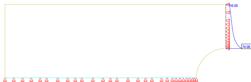
Figure 46.4: Maximum Stresses \sigma_{xx,max}
