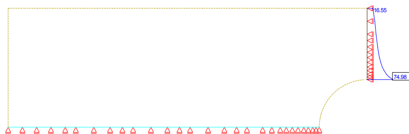
Figure 4: Maximum Stresses \sigma_{xx,max}
